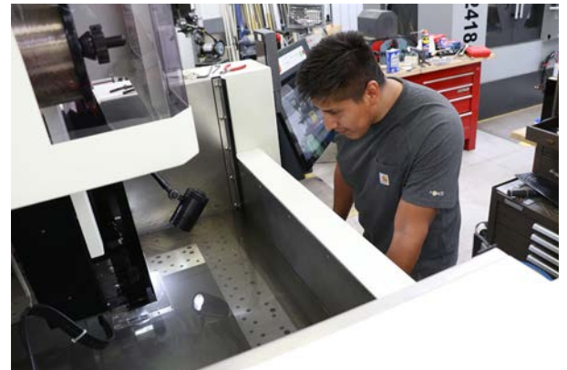
Shane Tsosie programs NTU's EDM machine to make a cut of a 3D metal print. The machine uses electrical discharge utilizing a copper wire to make the precise cut.
