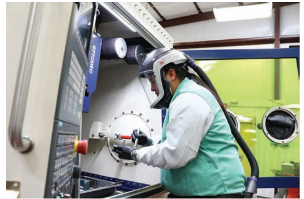
Joshua Toddy extracts a 3D metal print from NTU's Optomec LENS MTS 500 HY CA system. Toddy runs the machine for NTU's Center for Advanced Manufacturing.
